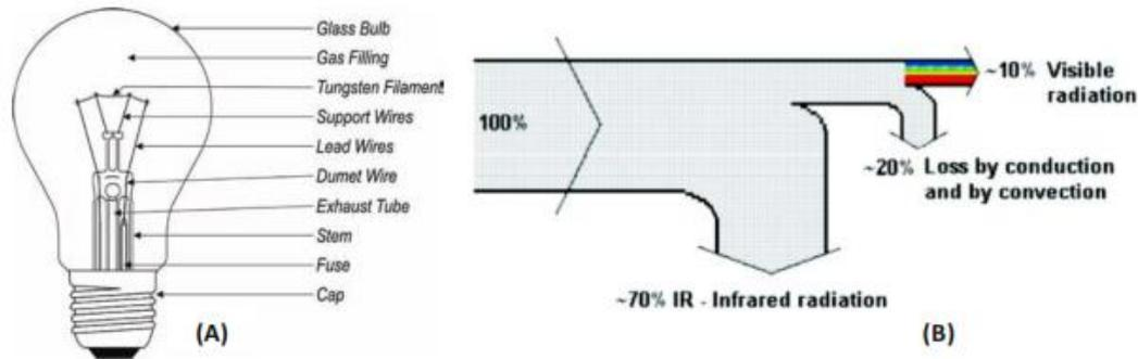
Figure 8.3 Incandescent Lamp and Energy Flow Diagram
