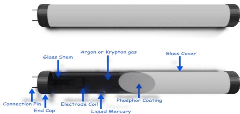
A fluorescent lamp has changed over electrical energy into useful light energy to a great deal more proficiently than incandescent lamps. The normal luminous viability of fluorescent lighting frameworks is 50 to 100 lumens per watt, which is a few times the adequacy of incandescent lamps with equivalent light yield.
