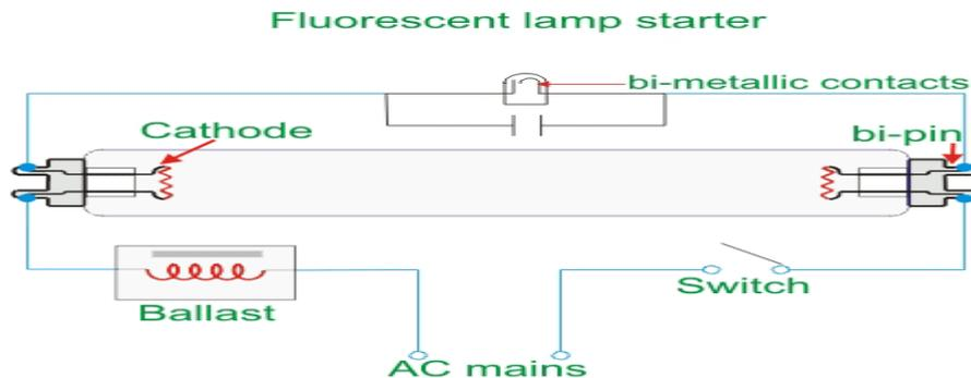
Here we connect one ballast, and one switch and the supply is series as shown. Then we connect the fluorescent tube and a starter across it.
