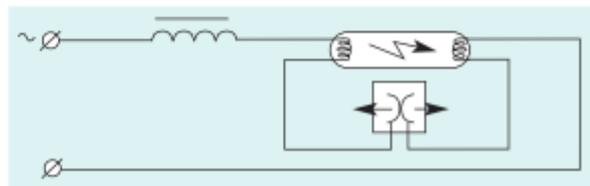
In addition to the ballast and the starter most fluorescent lamps circuits have a capacitor connected across the supply terminals to ensure a high power factor for the circuit.
