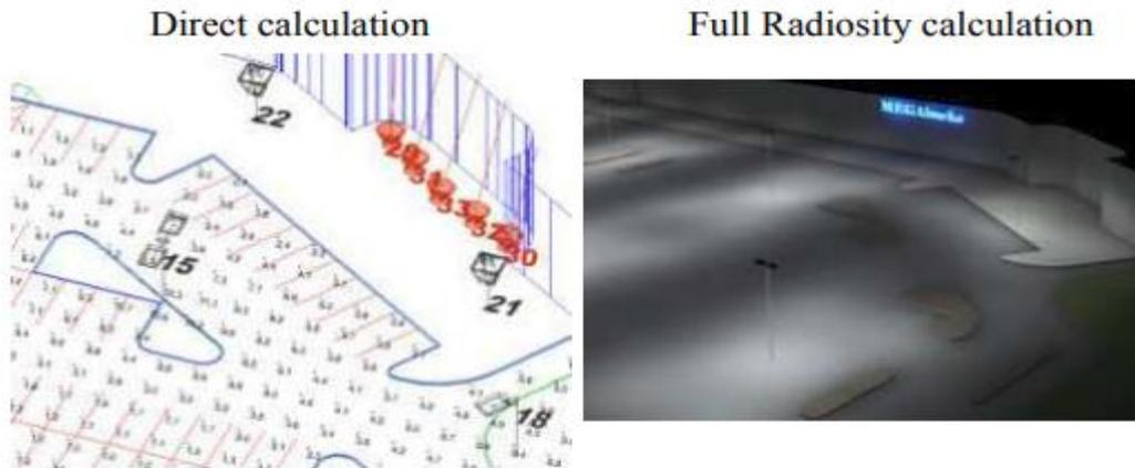
Lighting calculations and simulation in Revit BIM using ElumTools
