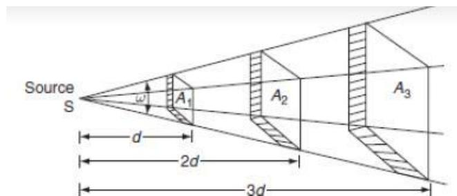
Let, 'S' be a point source of luminous intensity 'I' candela, the luminous flux emitting from source crossing the three parallel plates having areas  $A_1$ ,  $A_2$ , and  $A_3$  square meters, which are separated by a distances of  $d$ ,  $2d$ , and  $3d$  from the point source respectively as shown in Fig.
