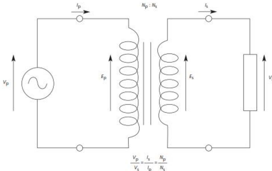
**Figure 5.10** A circuit diagram for a transformer
