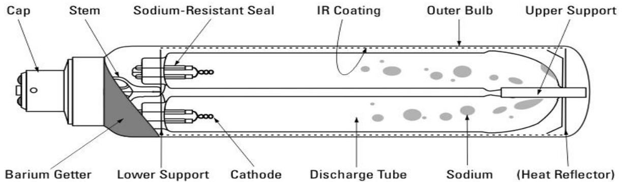
**The constructional features of the LPSV lamp are given below:**
