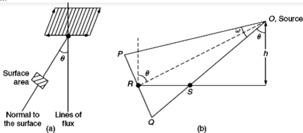
Let us assume that the surface is inclined at an angle ' $\theta$ ' to the lines of flux as shown in Fig. (a)
